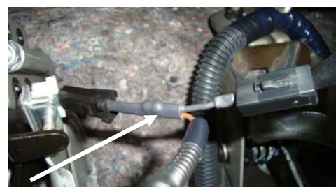
Park Brake connection behind pedal
