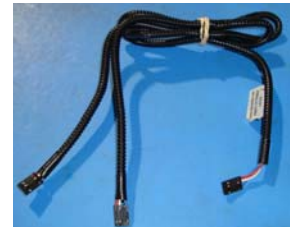
"Y" Harness. Single end on right connects to LED panel, double ends on left connect to MIM & GTWY modules.
