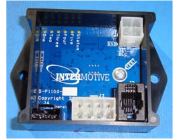
MIM401 - Merlin Interface Module transmits vehicle data to Merlin system.
