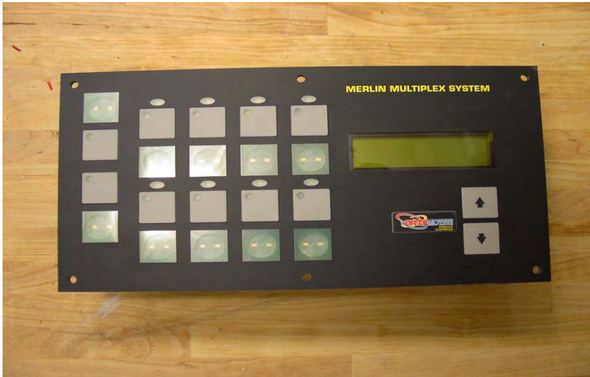
• Figure 2: Intelligent Switch Panel
